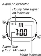
When the Daily Alarm is turned on, the alarm sounds for 20 seconds at the preset time each day. When the Hourly Time Signal is turned on, the watch beeps every hour on the hour.
