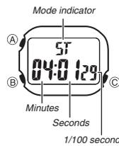
The Stopwatch Mode lets you measure elapsed time, split times, and two finishes. The range of the stopwatch is 59 minutes, 59.99 seconds.
